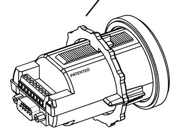
The gasket around the ring of Your Meter should provide an adequate seal against moisture. If a sealant is used be sure it is **silicone** so that the meter may be removed without damage.
